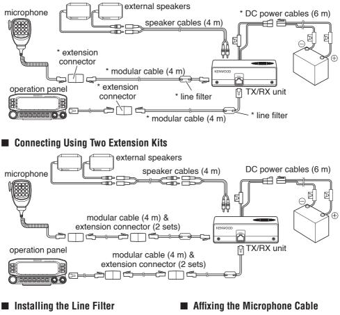
Install the line filter approximately 3 cm from the connector which attaches to the TX/RX unit.
