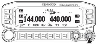
Pressing **[PF2]** allows you to switch the operating band between bands A and B, while maintaining the original band as the transmit band.
