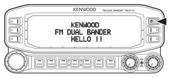
Press the [**b**] switch again to switch the transceiver OFF.
